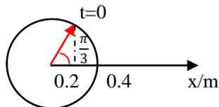
21.解: (1)  $A = 30\text{cm} = 0.3\text{m}$     $T = 5\text{s}$     $\omega = \frac{2\pi}{5}\text{rad/s}$
